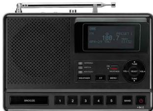
The CL-100 has a graphic LCM (128 \* 64 Pixels Graphic) LCD module with excellent display quality and wide viewing angle. It can scroll LCD display of S.A.M.E. event information. In addition, the CL-100 has dimmer and contrast control adjustment for viewing the display in the dark.
